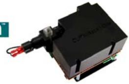
The DLP NIRscan is a complete evaluation module (EVM) to design a high performance, affordable near-infrared spectrometer. The EVM features the DLP4500NIR DMD and is optimized for material sensing in the 1350 – 2450nm wavelength range.
