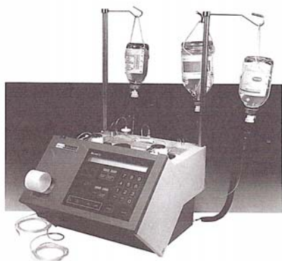
FIGURE 18.1 A general view of the Betalike, the artificial pancreas developed and marketed by Esacontrol (Genoa, Italy).
